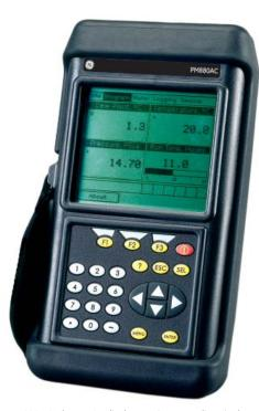
The PM880 AC's large LCD displays moisture readings in dew point (°C or °F), ppm $_{\nu}$ , ppm $_{\nu}$ , lb/MMSCF (natural gas), and a variety of other unit options in graphic or alphanumeric formats.
