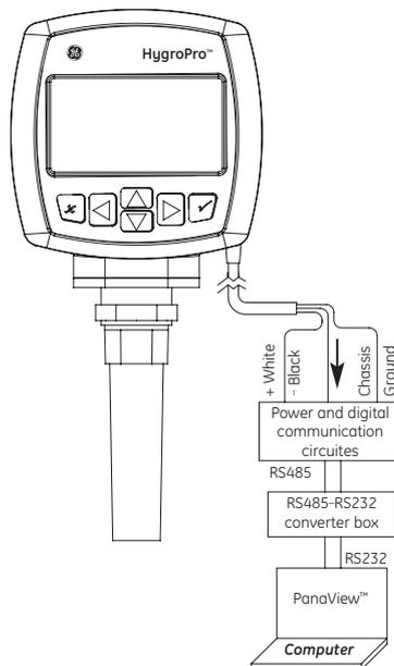
*Digital communications wiring connection
