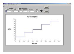
Prostep software enables "ramp and soak" humidity and temperature profiles to be loaded into the Humilab. Prostep also features data logging. The chamber conditions are recorded as time-based ASCII data, which can be opened in spreadsheet programs such as Excel.
