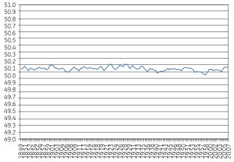
The graph above was produced with data from the Humilab. The calibration system provides stability of better than  $\pm 0.2\%$  RH.
